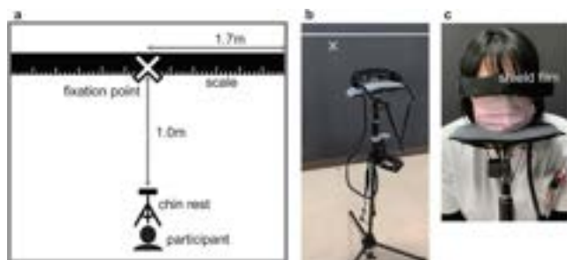
Fig. 3 Examination conditions. a Layout of the examination. b Photograph of the actual examination condition. c Use of a shield film to shield the outer vision, except when the night-vision aid is powered off
