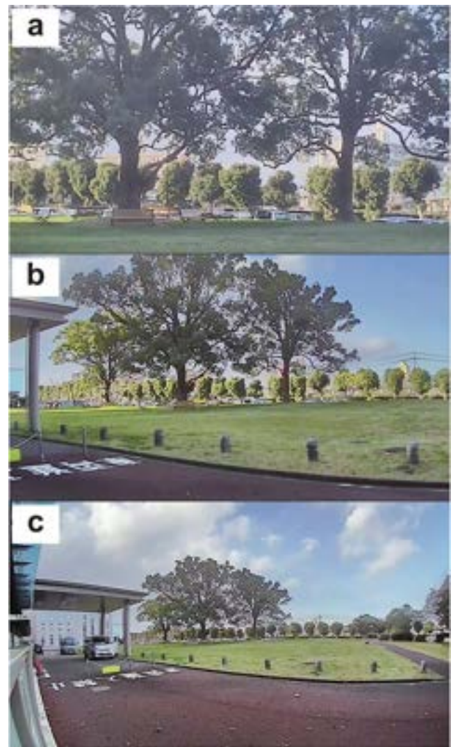
Fig. 2 Actual images obtained using each lens at the same position. a Standard-angle lens. b Middle-angle lens. c Wide-angle lens
